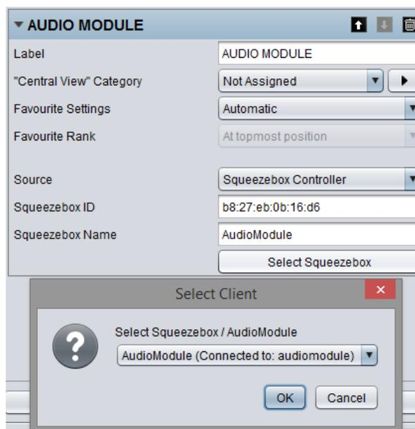
Figure 137: Multimedia element - Squeezebox Controller configuration
