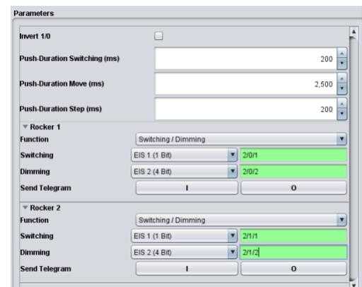
Figure 190: Sending KNX Parameters
