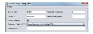
Figure 185: EnOcean Device Configuration
