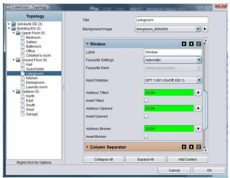
Figure 122: configuration of window contact
