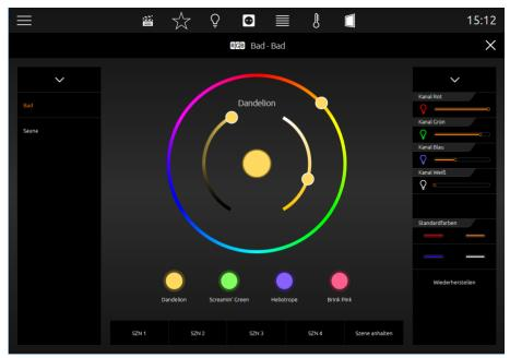
Figure 124: extended element view of RGB control
